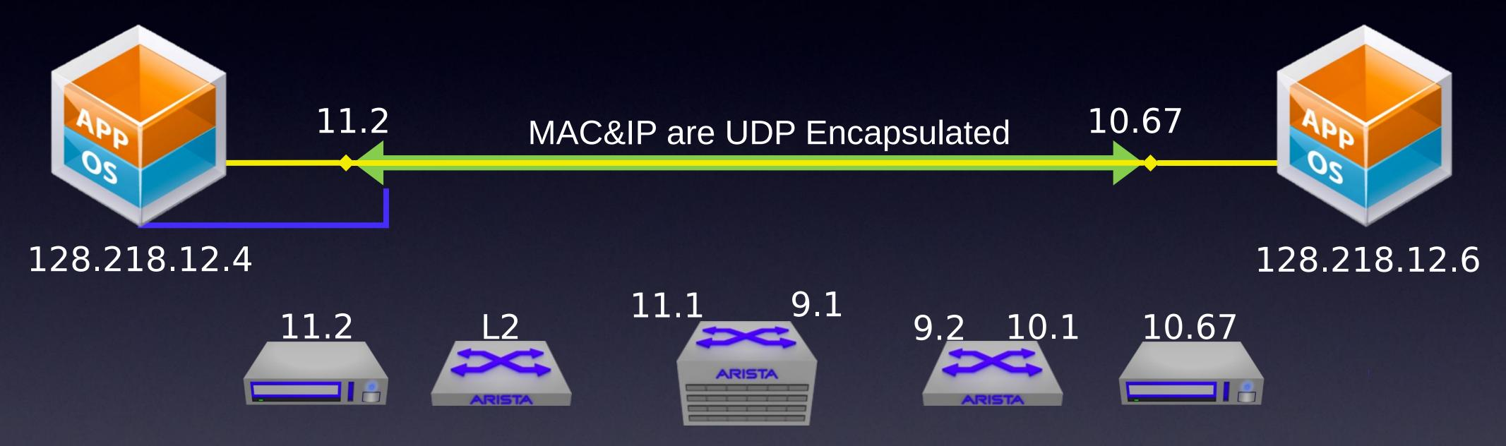
Encapsulation is transparent to traditional switch/router nodes
